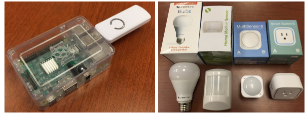
Figure 3: A Raspberry Pi with Z-Wave Dongle (left); Example of Z-wave Compatible Smart Devices (right)
